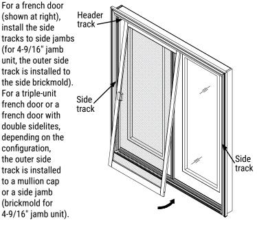
NOTE: For Jamb widths between 4-9/16" and 5-1/2", add a ½" x 1" Spacer (not supplied) to the vertical Brickmold edge. This will fill the gap between the C-Channel and the Brickmold. The Spacer provides secure mounting for the C-Channel screws. (shown at right)
