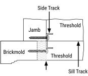
For a double patio unit with one swinging door, one side track is installed to a jamb (brickmold for 4-9/16" jamb unit). For triple patio unit with one swinging door, depending on the configuration, side track may be installed on a mullion cap or a side jamb (brickmold for 4-9/16" jamb unit). For the above patio units with single swinging door, screen door is installed on the outer track.
