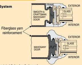
\*Maximum protection is achieved only when the door system is installed and caulked properly.
